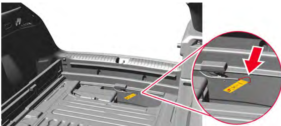
Cut-out connection in the Q4 e-tron luggage compartment under the luggage compartment floor at the rear cross panel. The yellow tag indicates the cut-out connection.
