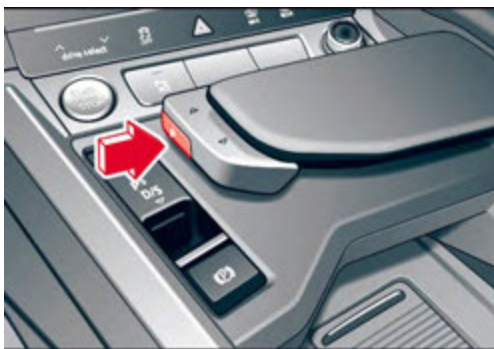
Vehicles with an automatic gearbox without a selector lever: press the “P” button
