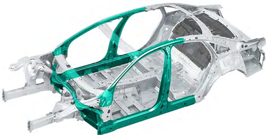
Body with reinforced passenger compartment
