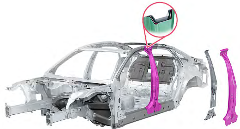
B-pillar with multi-shell structure
