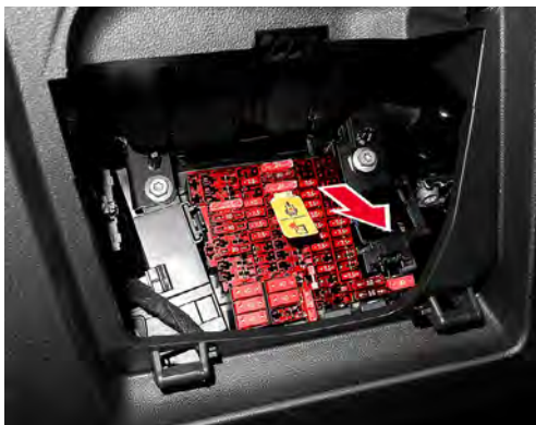
Emergency cut-out connection, fuse carrier
