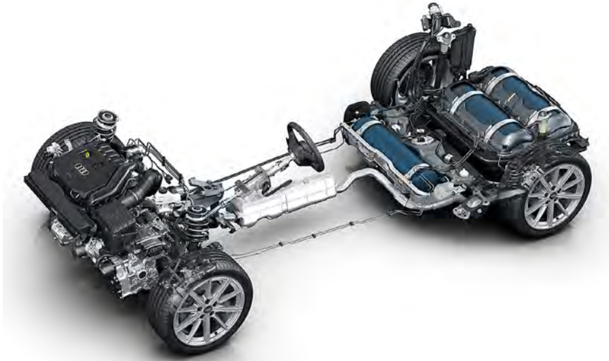
Audi A3 g-tron with 3 gas tanks
