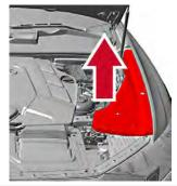
Trigger device that disconnects high voltage
