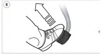
Electronic emergency gearbox release is only possible if the engine does not start, but the starter motor rotates.
