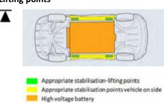
Use caution to ensure you never come into contact with the high voltage battery or other high voltage components while lifting or manipulating the vehicle.
