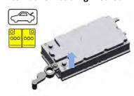
The vehicle power system can be shut down normally. Power off and disconnect the negative cable of 12V lowvoltage battery.
