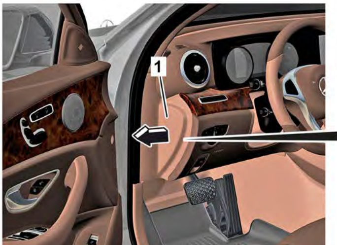
Remove cover (1) of fuse box / Cut line at marked location (2)
