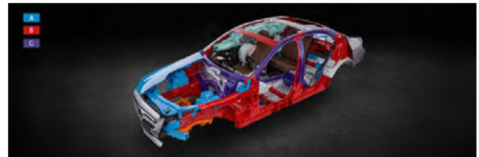
Overview of materials using E-Class Sedan (W213) as an example.
