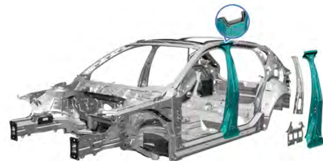
B-pillar with multi-shell structure
