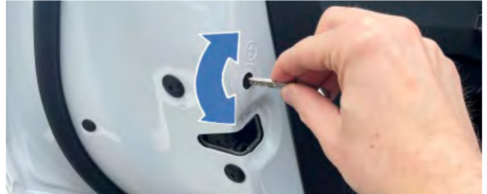
Deactivate the childproof lock mechanically using the key.
