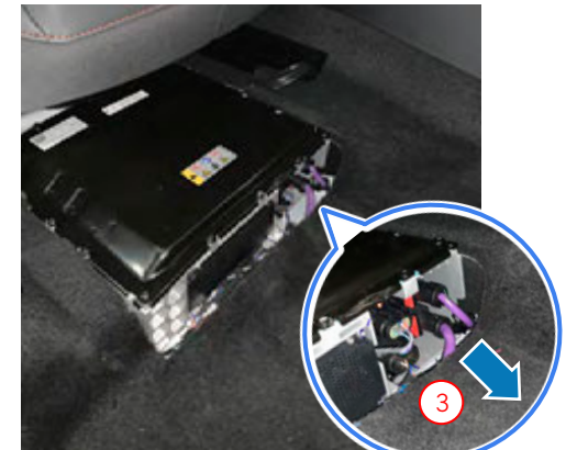
Disconnecting the 48-volt vehicle electrical system in mild hybrid vehicles (MHEV).
