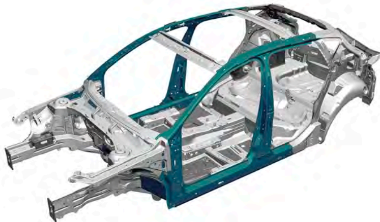
Body with reinforced passenger compartment
