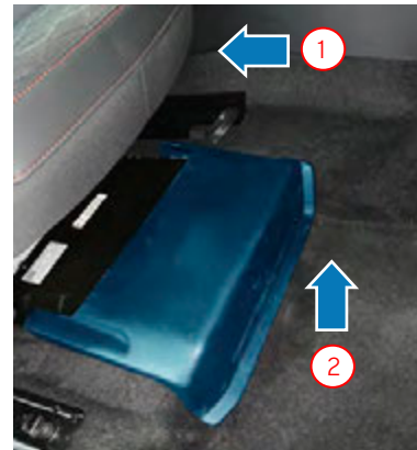
Disconnecting the 48-volt vehicle electrical system in mild hybrid vehicles (MHEV).
