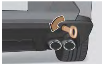
Fastening of the rear towing eye
