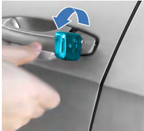
Unlock turning the key
