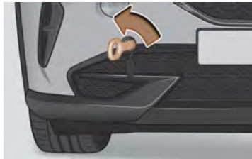
Fastening of the front towing eye
