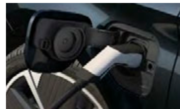
Charging socket lid on the LEON eHybrid (plug-in hybrid)
