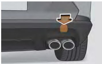
Access cover to the rear towing eye
