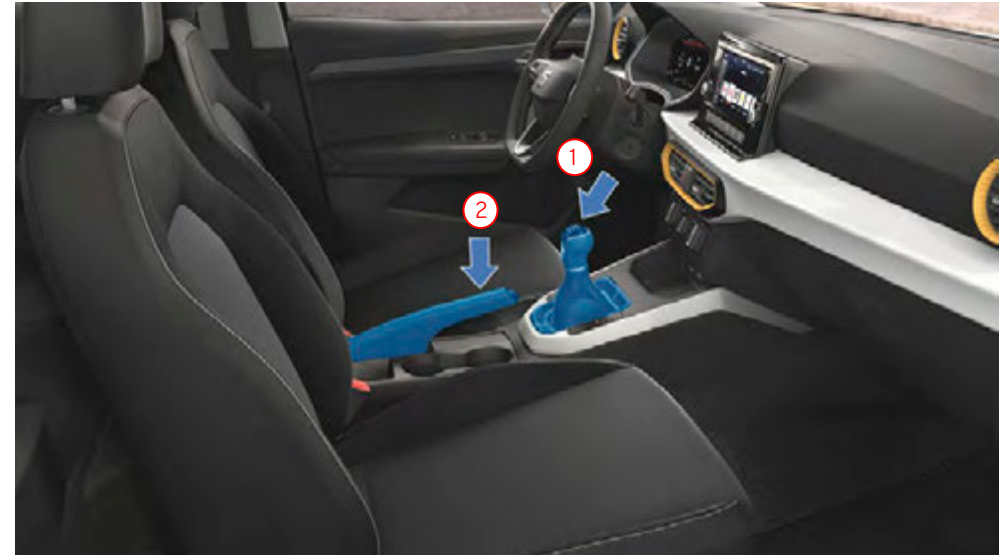
Vehicle with manual drive train: Put the gear lever into neutral (1) and apply the handbrake (2).
