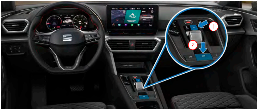
Vehicles with automatic gearbox without selector lever: press P button (1) and activate the electric handbrake (2).
