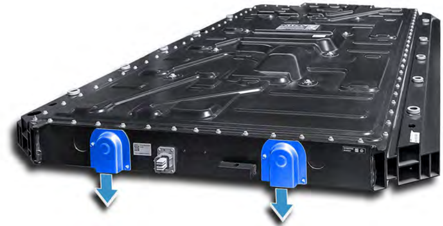
High-voltage battery with vents pointing downwards
