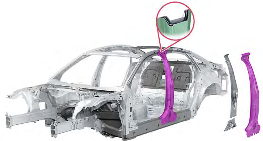
B-pillar with multi-shell structure
