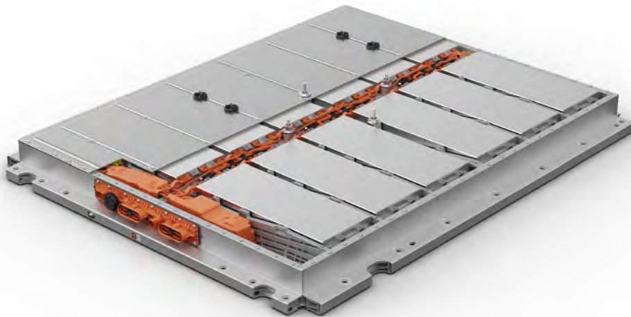
The high-voltage battery of ID. family
