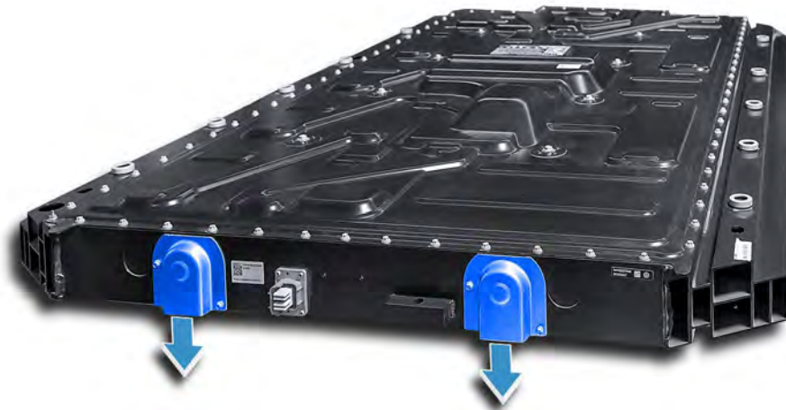
High-voltage battery with vents pointing downwards
