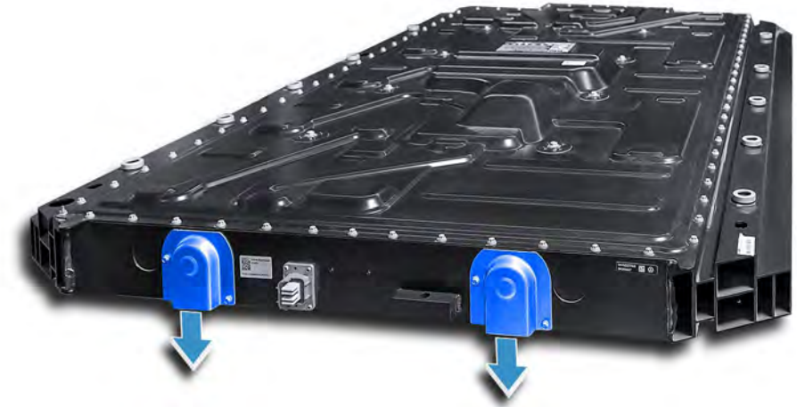
High-voltage battery with vents pointing downwards
