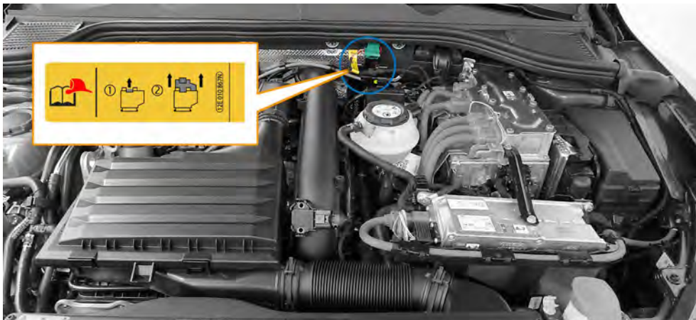
Cut-out connection in the vehicle front end of a hybrid vehicle (example Golf GTE, from 2020 onwards).
