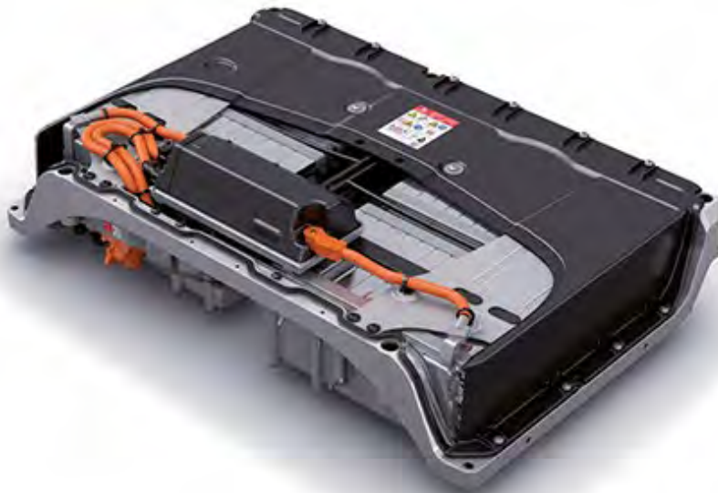
The high-voltage battery of the Passat GTE
