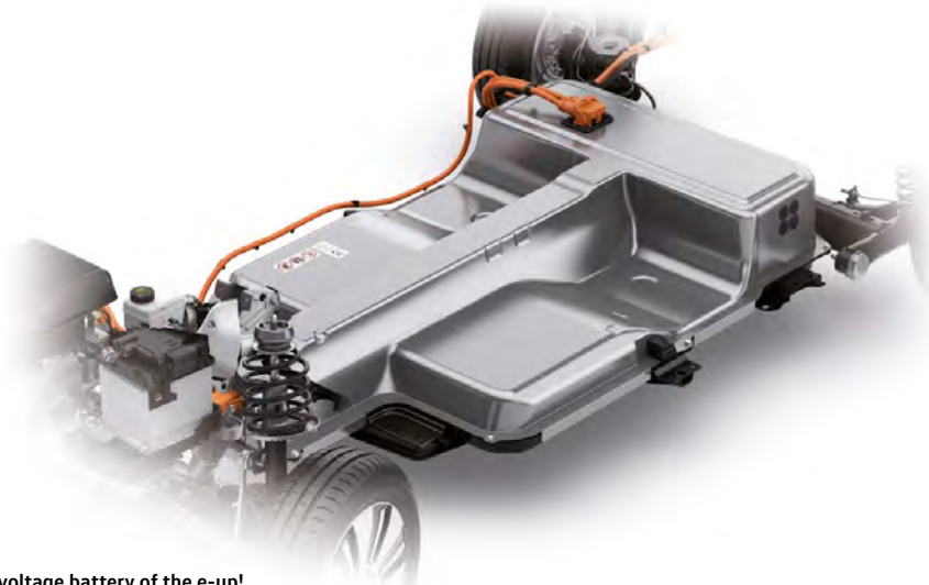
The high-voltage battery of the e-up!
