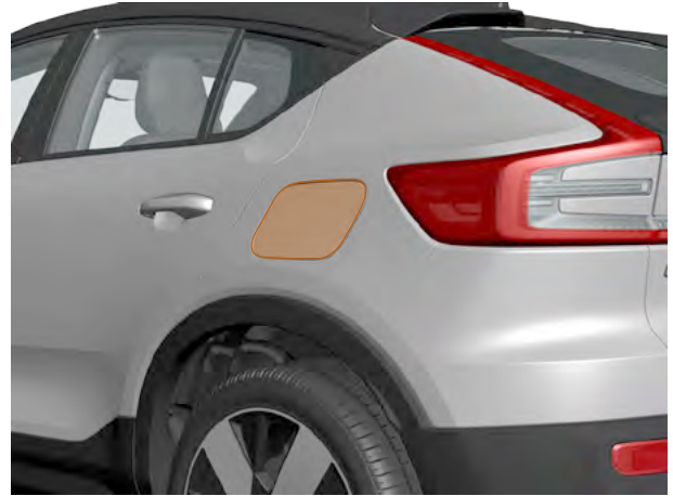
The charging lid is placed on the driver's/left side of vehicle.
